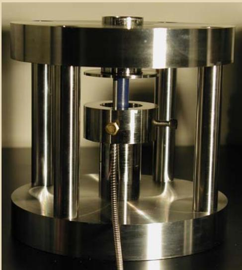
*While accurately controlling temperature, platen separation is measured using a laser device. Over time (ranging from hours to days) longitudinal sample deformation is observed in response to applied stress. Several experiments, with different loads, may be utilized to comprehensively map strain rate in response to stress. In this way, pitch rheology (deformation due to stress) may be understood and used to quantify “hardness” and related polishing characteristics.*
