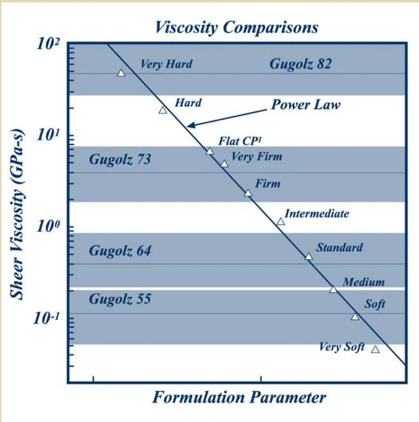
*For comparisons, we have extensively measured the viscosity of various natural polishing pitches. Although competitive pitches cover broad ranges, average viscosity, and likely ranges for important Gugolz pitches, are shown here as blue bands (with center lines for the average).*
