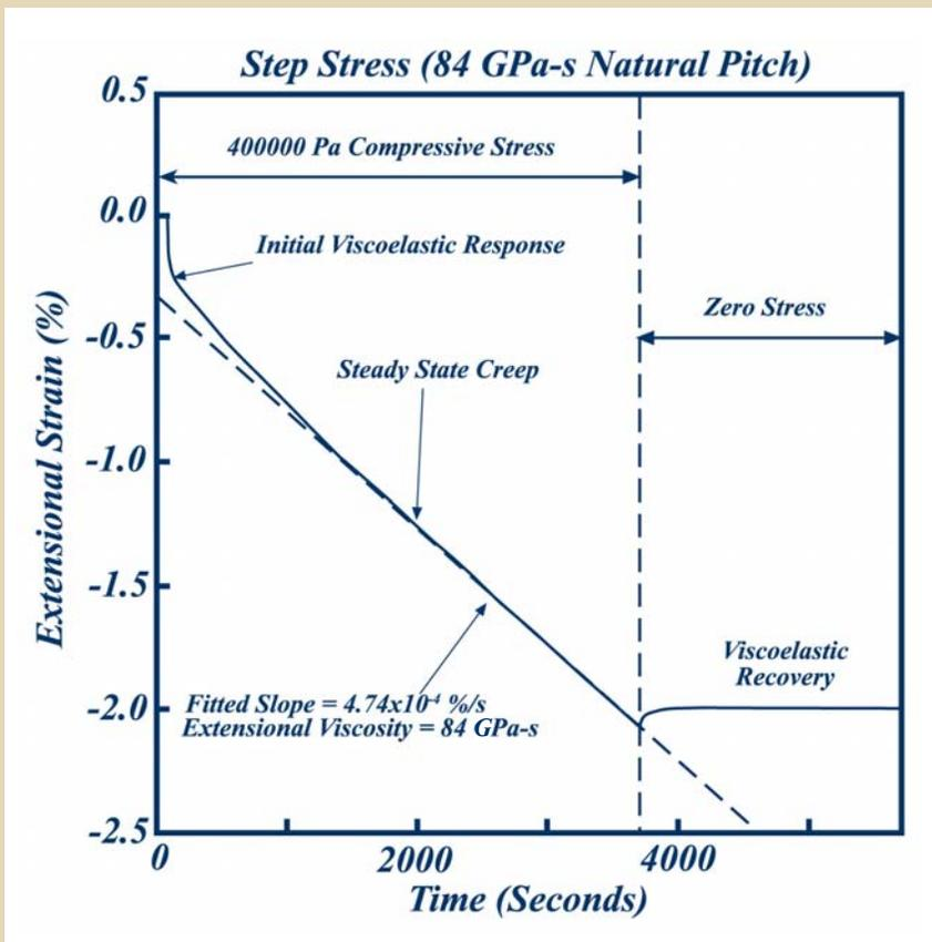
*In a typical rheological experiment, deformation of a sample (shown here as a percentage change in length) is measured following the application of stress. The incredible accuracy of our technique allows observation of initial viscoelastic effects and subsequent steady state creep or flow. Even slight viscoelastic recovery of the pitch, following removal of stress, may be measured in detail.*
