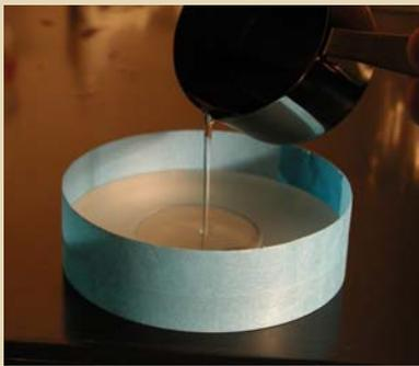
**How is Acculap™ heated and poured?** *Acculap™ pitches are all designed to be easily poured at a temperature of 135°C (similar to natural pitches). Odor is minimal while the material is non-toxic and highly stable against drying. Consequently, Acculap™ processes without the odor, health concerns, and drying sensitivity of natural pitches.*
